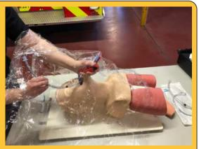
The above figures are examples of the clear plastic shroud. The shroud may be placed directly over the patient's head and neck while the EMS clinician managing the airway does so with the airway management device and their hands UNDER the shroud.
